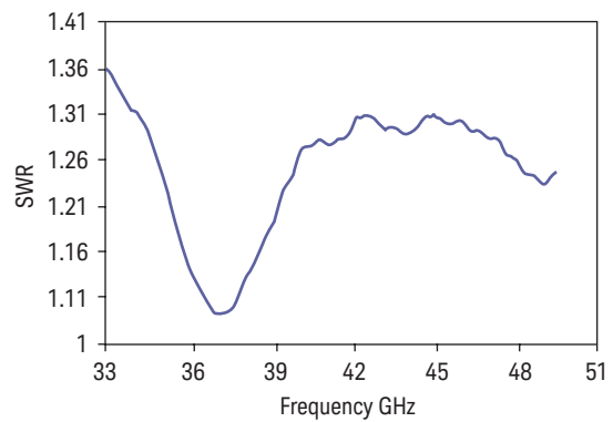
Typical SWR, 33 to 50 GHz (25 ± 10 °C) for N8486AQ power sensor
